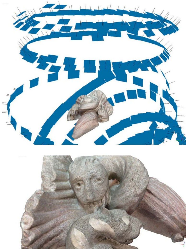
Figure 42 Top row: Orientation of cameras calculated. Bottom row: Dense point cloud generated [124]
